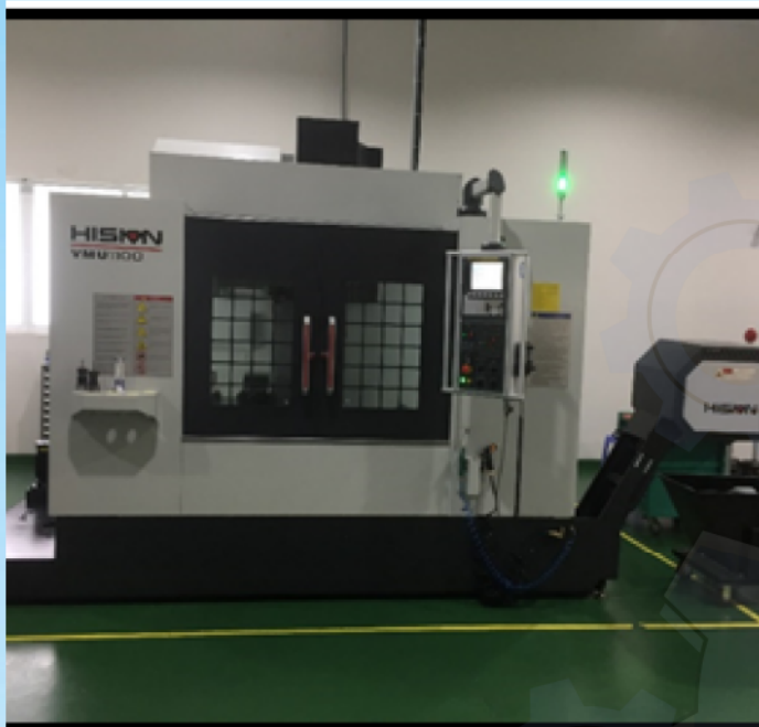
Máy phay CNC/ Machining center : HAITIAN Vertical machining center
